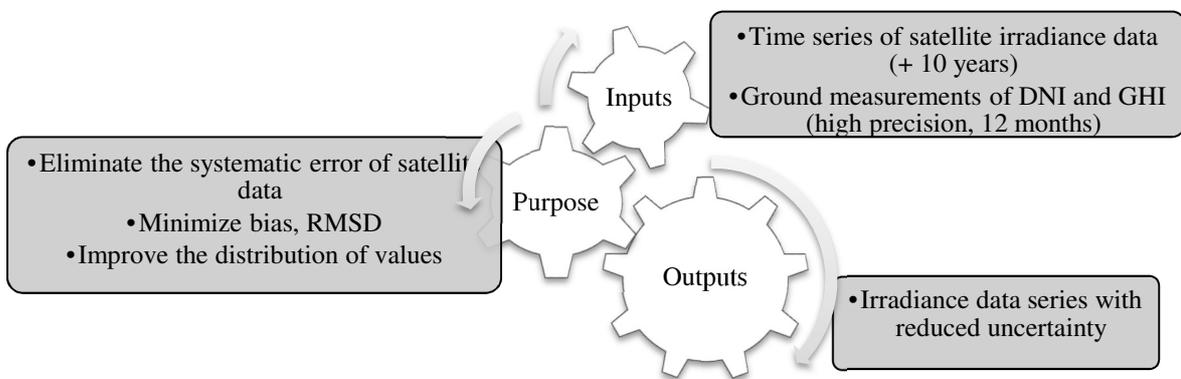
**FIGURE 1.** Principle of statistical approach of local calibration
