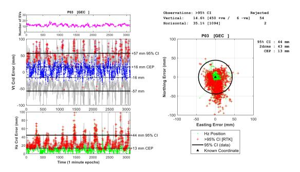
Figure 7: Height [blue dots] and horizontal [green dots] positions for the GPS + Galileo + BDS constellations, Trimble R10 [GEC]. The grey line represents the R10 computed 95% CI (formal) error. The red "+" are outlier positions that lie outside the 95% CI for which there are 15% (vertical, total 450) and 35% (horizontal, total 1094). There was 54 / 2 rejected vertical / horizontal positions being greater than 100 mm error.
