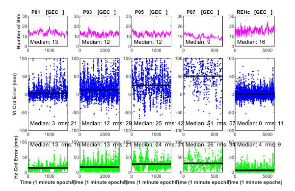
Figure 8: Summary plots for the sites P1, P3, P5, P7 and REH. Shown are the median number of satellites (top row), median coordinate error and rms for the vertical (middle row) and horizontal (bottom row) coordinate error.
