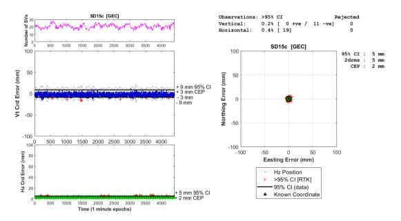
Figure 5: Height [blue dots] and horizontal [green dots] positions for the GPS + Galileo + BDS constellations, Trimble R10 [GEC]. The grey line represents the R10 computed 95% CI (formal) error. The red "+" are outlier positions that lie outside the 95% CI for which there are 0.2% (vertical, total 11) and 0.4% (Horizontal, total 19). There were no rejected observations (>100 mm error).
