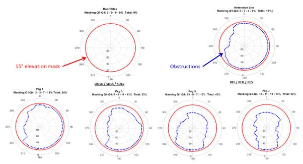
Figure 4: Sky visibility plots. The roof sites (OUSD, SD14, SD15) did not have obstructions above 15° (and the instrument elevation mask was set to 15°). The reference sites REF, REH and RES had masking above 15° of 19%, while the pegs P1, P3 P5 and P7 had increasing masking of 24%, 23% 43% sand 52% masking.
