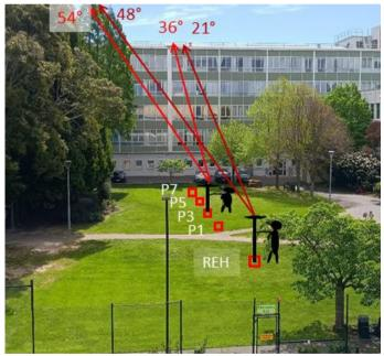
Figure 2: Location of the survey marks showing the increase in sky visibility masking towards the building (background) and the tall trees on the LHS. The building is approximately 18 m high. The marks REF/REH and RES are the same mark.
