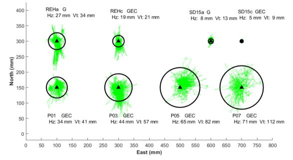
Figure 9: Plots of horizontal position for the sites reference site REH (G and GEC constellations); the roof sites SD15 (G and GEC constellations); and the ground sites P1, P3, P5, P7 (GEC constellations only), The black circle represents the 95% CI horizontal coordinate uncertainty, and the 95% CI numerical uncertainties are given for both the horizontal and vertical coordinate components.
