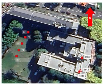
Figure 3: RTK positioning error network. The GNSS base station is on the roof of a three-floor building. The survey marks OUSD, SD14 and SD15 have no sky visibility masking while the survey marks at ground level (REH, P1, P3, P5 and P7) all have some level of sky visibility masking.
