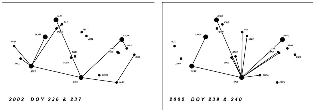
Fig. 4 The independent baselines used for GPS data processing in KARKONOSZE 2002 network
