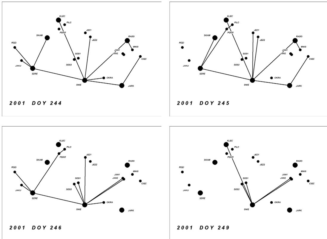
Fig. 3 The independent baselines used for GPS data processing in KARKONOSZE 2001 network
