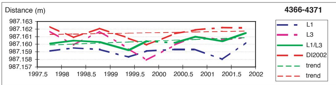
Fig. 8. The distance variation between points 4366-4371 measured by GPS ( $L_1$ ,  $L_2$ ,  $L_1/L_2$ ) and by electronic distance meter DI2002.
