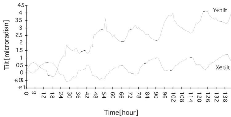
Fig. 7. Tilt caused by the transpiration of the trees recorded at the point D2 from 11.08.1998 till 17.08.1998
