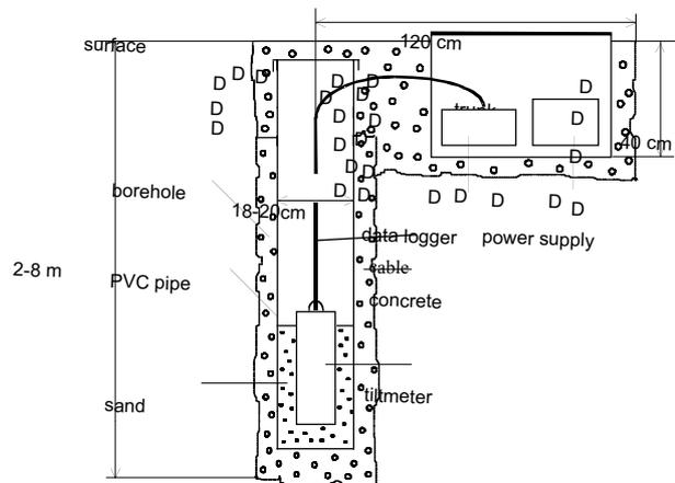
Fig 1. Installation of Model 722 tiltmeter in the borehole
