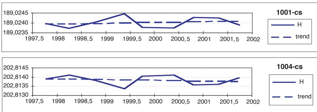
Fig. 9. The height variations of the two endpoints of the leveling line.
