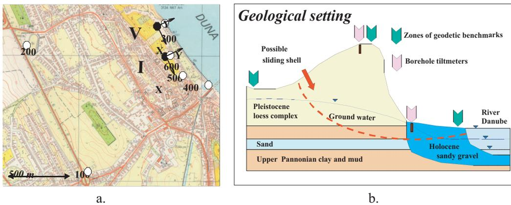
Fig. 10. Map of the test site in Dunaföldvár (a), geological structure of the high bank
