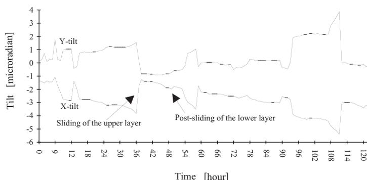
Fig. 6. Landslides recorded at the point D2 from 24.03.1998 till 29.03.1998
