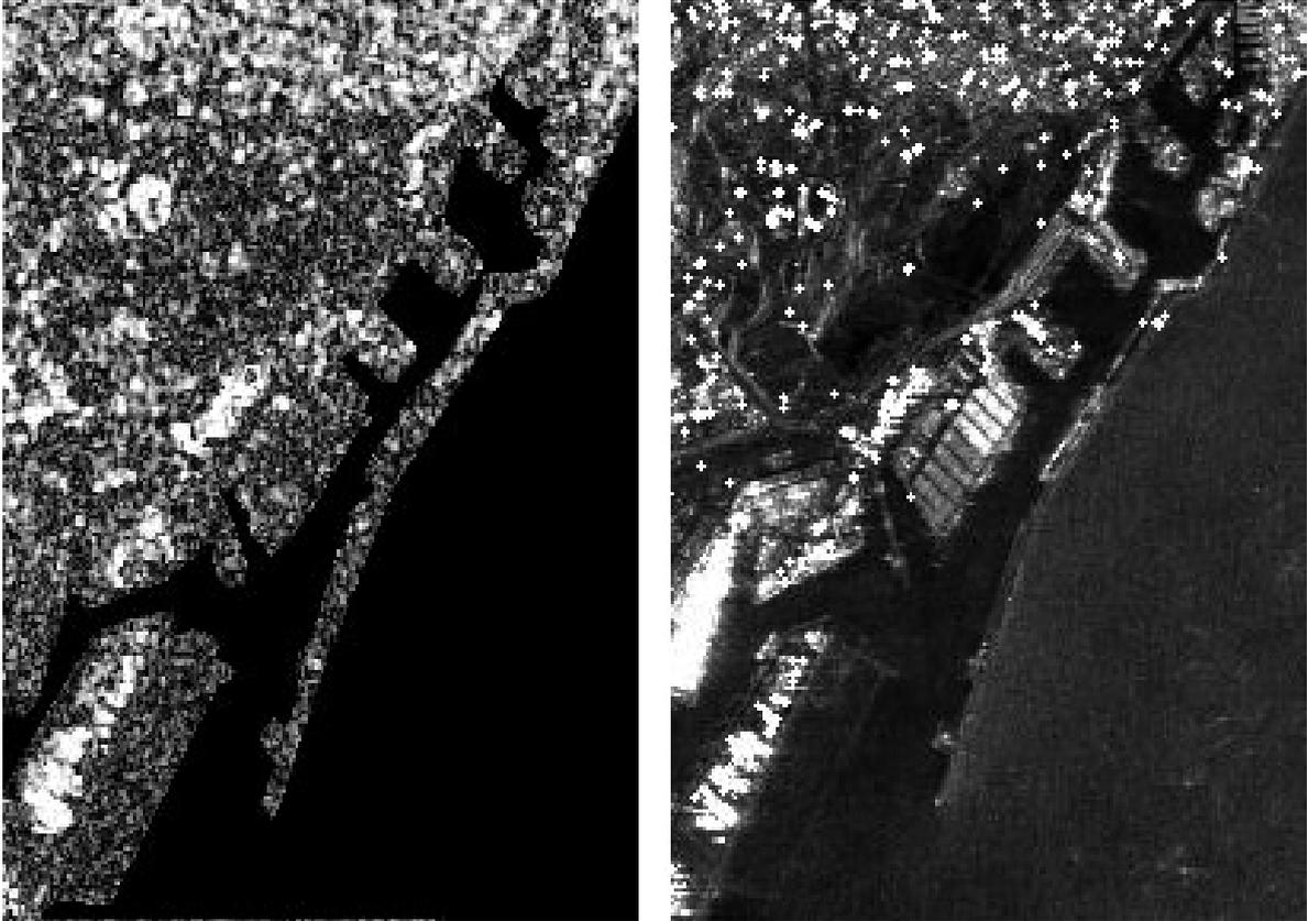
Fig. 2: Data availability for deformation control using two different DInSAR techniques: zoom on the framed area from Fig. 1. Coherence image (left side) and IPs estimated with a stack of 20 images superposed to the mean amplitude of the 20 SAR images. In order to ease the comparison, the coherence image was manually masked. There are 8916 pixels with coherence above 0.5, while only 422 IPs with  $D_A$  below 0.25.
