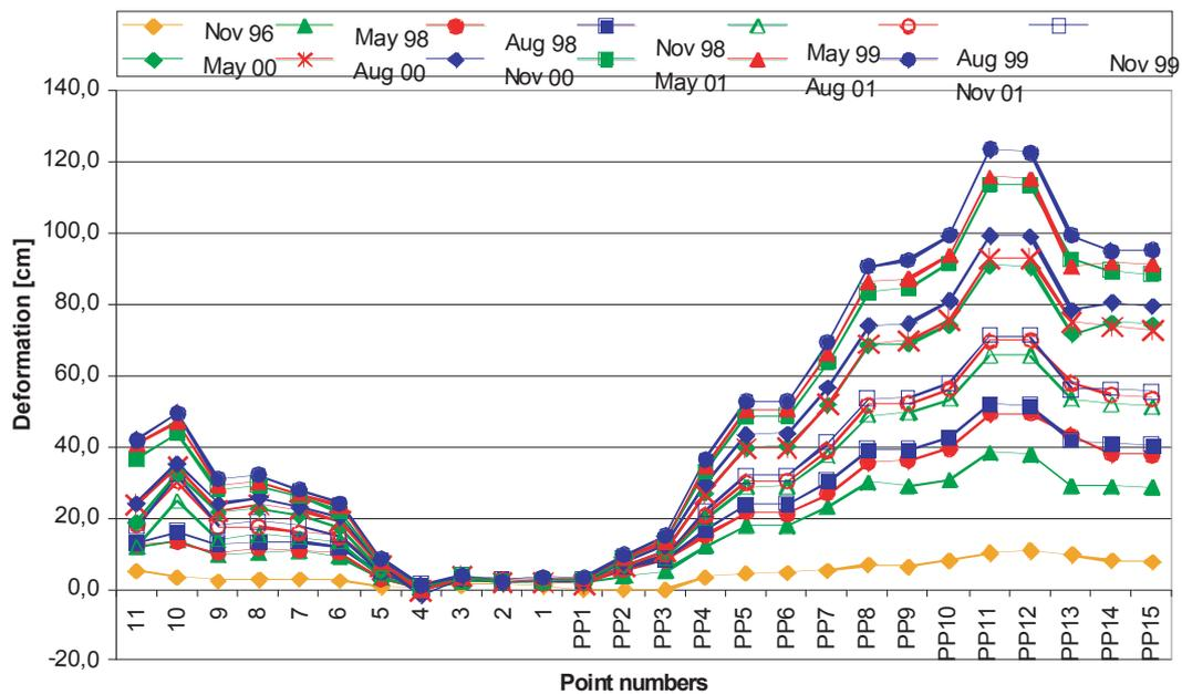
Fig. 6 Horizontal deformation characteristics of "Heumöser Hang", 14 epochs, GPS points (1-11) and the traverse
