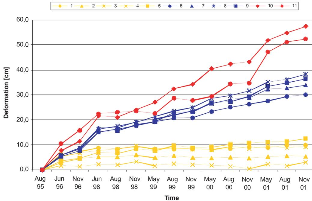
Fig. 4 Deformation analysis “Heumöser Hang” points 1-11, all epochs, horizontal displacements
