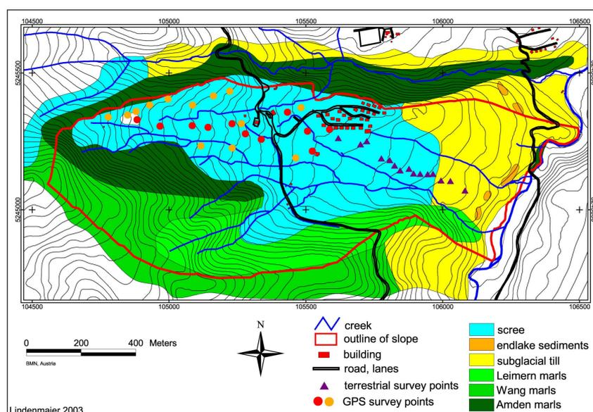
Fig. 2 Geology of the "Heumöser Hang", GPS and terrestrial measurement points
