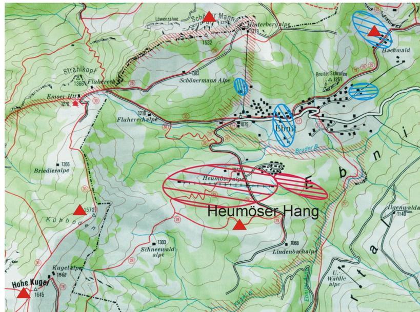
Fig. 1 Deformation network Ebnit with the reference points (triangle) and the 5 examination areas (“Heumöser Hang” red)
