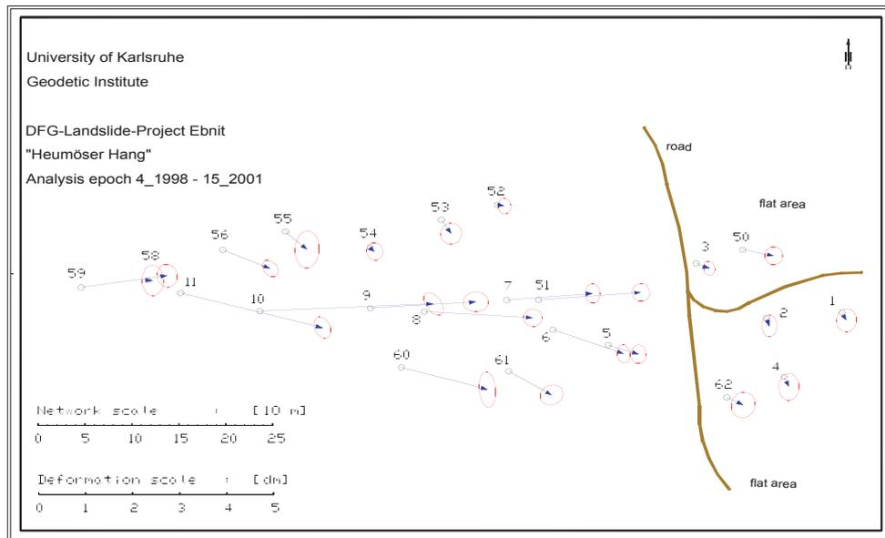
Fig. 5 Deformation analysis “Heumöser Hang” 4<sup>th</sup> and 15<sup>th</sup> epoch, points 1-11 and 50-62, horizontal displacement vectors with their confidence ellipses
