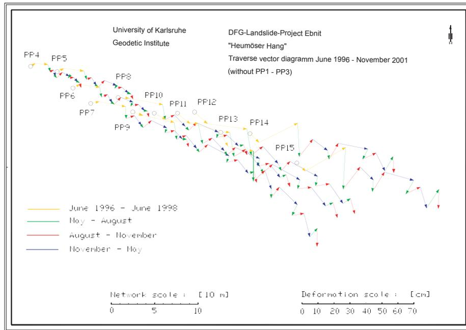
Fig. 6 Deformation analysis traverse (PP4-PP15), 14 epochs, horizontal displacements, vector diagram
