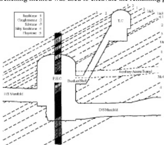
Fig. 2. Geology and relative position of the caverns.
