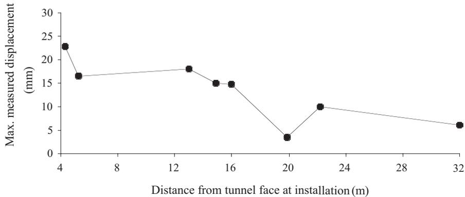
Fig. 4 Effect of face distance at installation on maximum measured displacement
