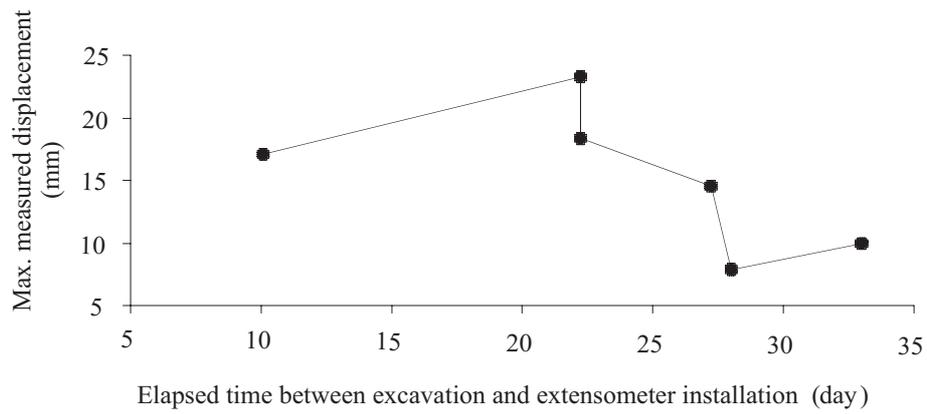
Fig. 5 Effect of time elapsed at installation on maximum measured displacement
