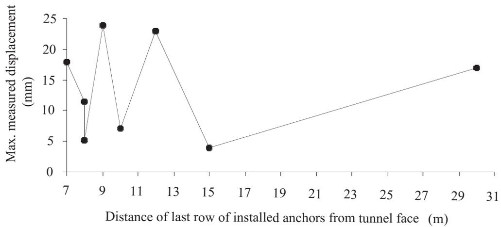
Fig. 6 Relationship between anchor installation and roof displacement
