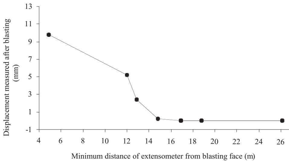
Fig. 7 Effect of face distance on measured displacement after blasting
