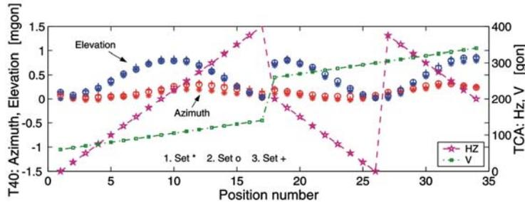
**Fig. 4.3:** Tripod movements for "set of angles": Leica, averaged AZ and EL values at the time of the direction observation, step width HZ 25 gon V 5 gon, 20 direction observations per position, 3 sets in succession
