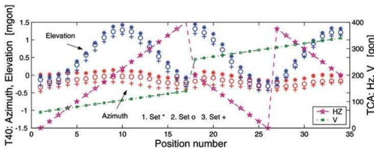
**Fig. 4.4:** Tripod movements for "set of angles": Crain, averaged AZ and EL values at the time of the direction measurement, step width HZ 25 gon V 5 gon, 20 direction observations per position, 3 sets in succession
