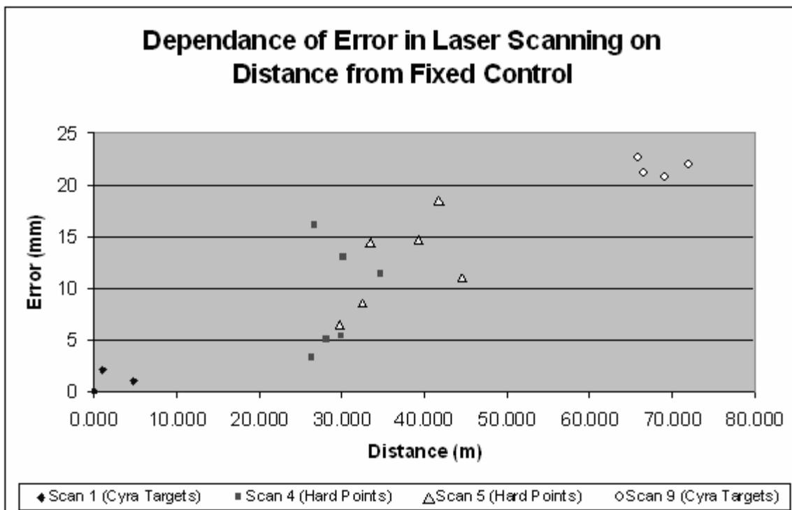
**Figure 5:** 3D Error vs. Distance
