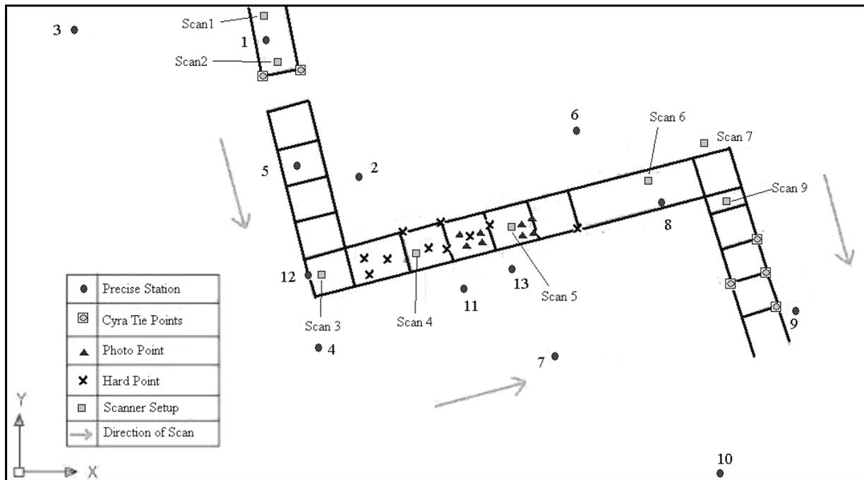
**Figure 1:** Overhead view of pipe rack section
