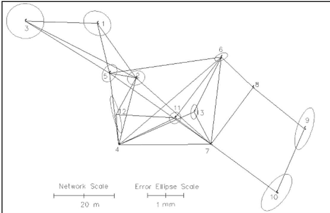
**Figure 2:** Network Geometry and Error Ellipses
