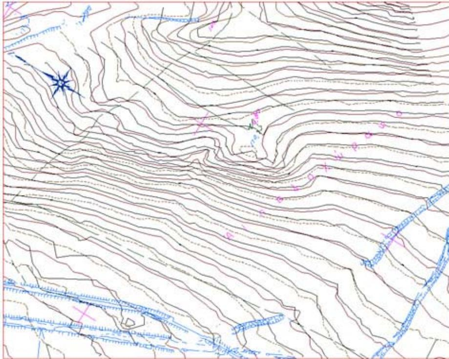
**Fig 4:** The two DTMs for the test area: a) obtained from GPS measurements (with black solid lines) b) derived from classical measurements (color lines).
