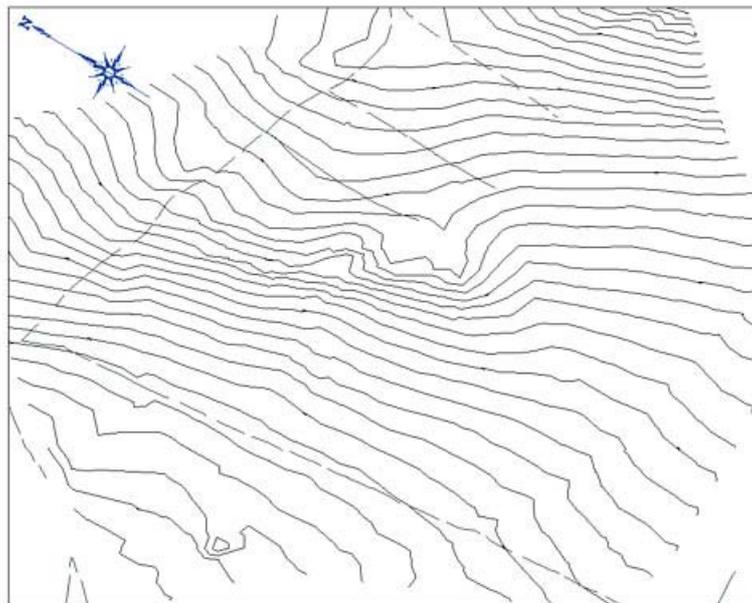
**Fig 3:** DTM obtained from GPS measurements for the same area
