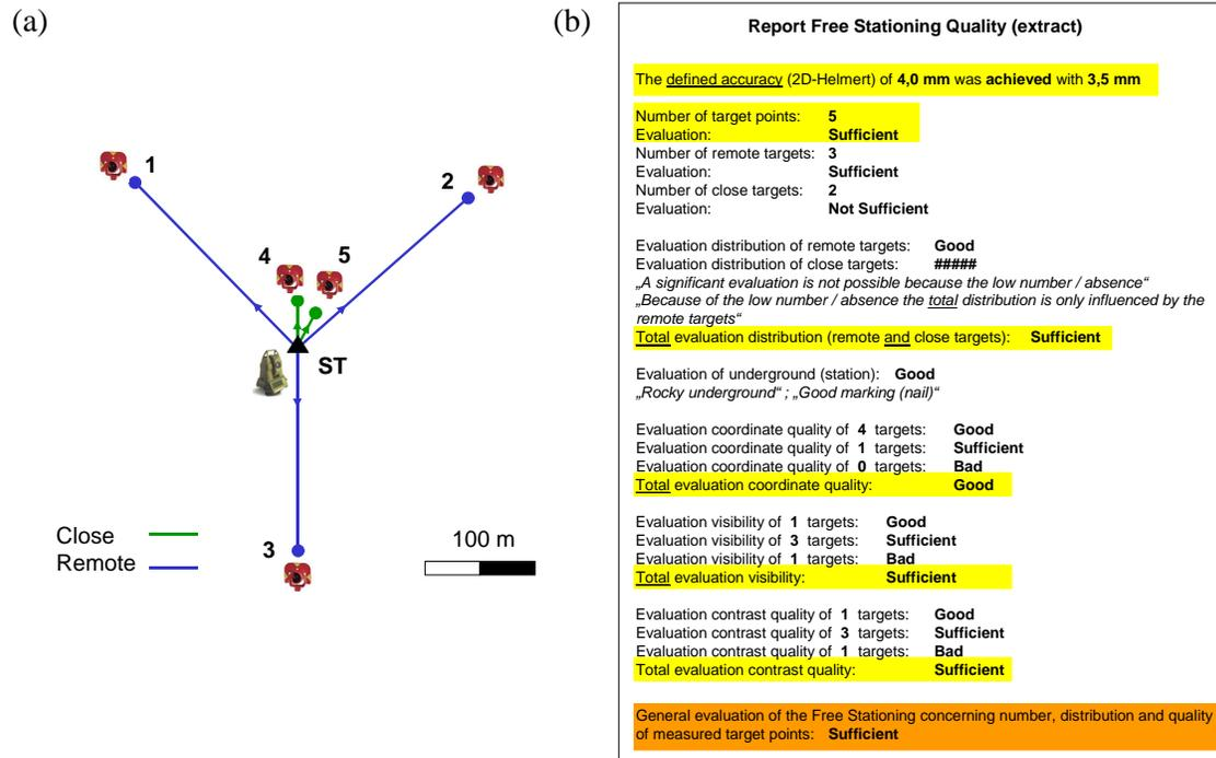
Figure 5 - (a) Simulation of a free stationing scenario and (b) extract of generated report
