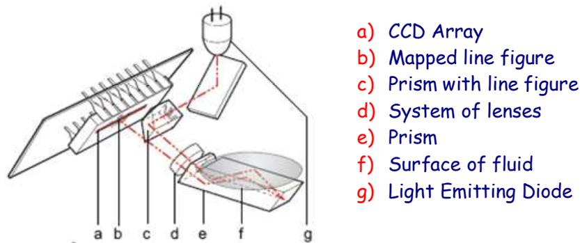
Figure 5 - Sensor components
