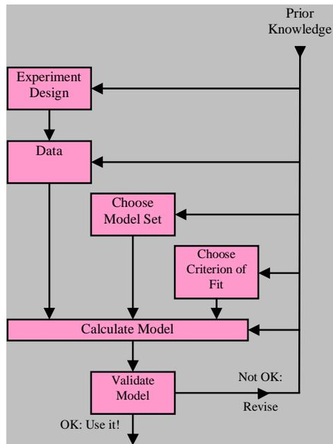
Figure 2 - The System Identification Loop (Ljung 1999)
