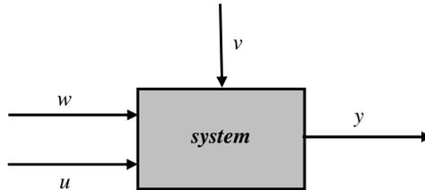
Figure 1 - A system with output  $y$ , input  $u$ , measured disturbance  $w$ , and unmeasured disturbance  $v$
