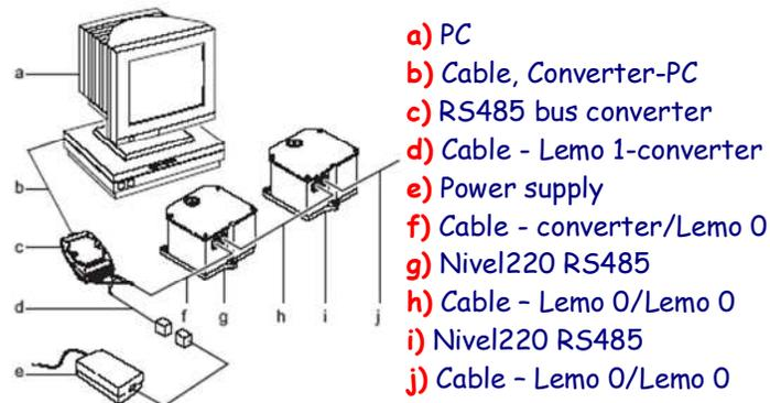
Figure 4 - Configuration of a Nivel 220
