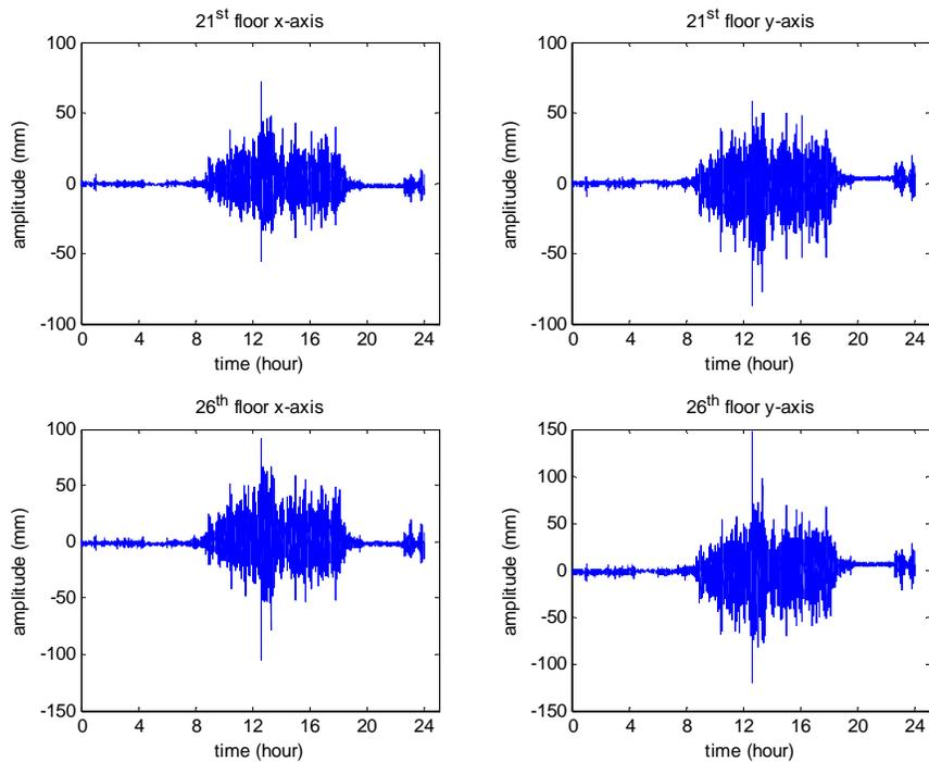
Figure 7 - Inclination sensor data collected in 23rd March 2006 during one day
