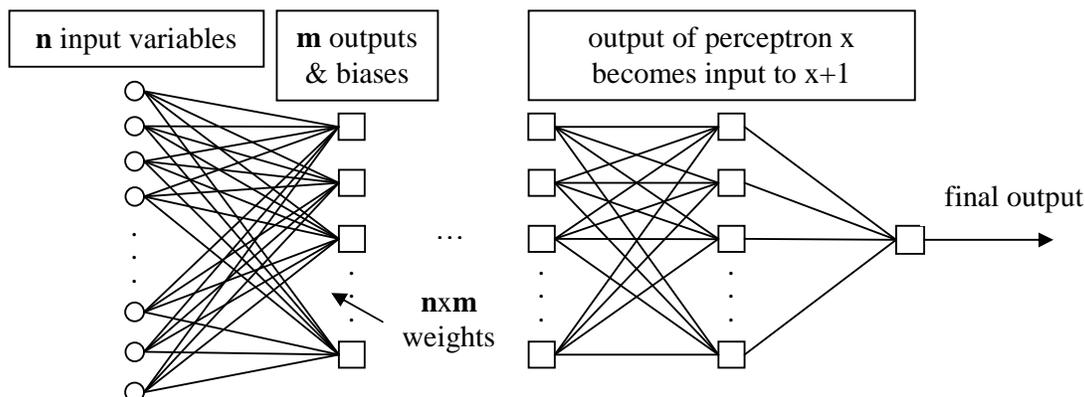
Figure 3 - Cascading Perceptrons or Multi-Layer Perceptron
