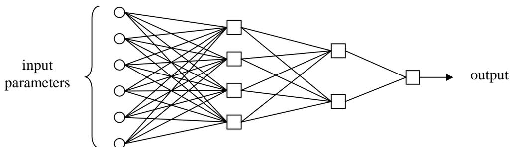
Figure 4 - MLP for deformation rate training & prediction
