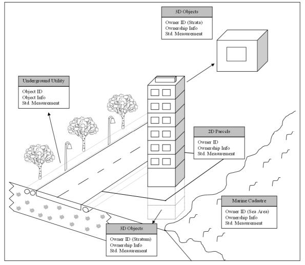
Figure 1: The anticipated schematic diagram of MPC
