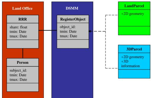
Figure 2. Adaptation of CCDM into Integrated 3D Cadastre Model for Malaysia where LandParcel and 3DParcel is part of RegisterObject
