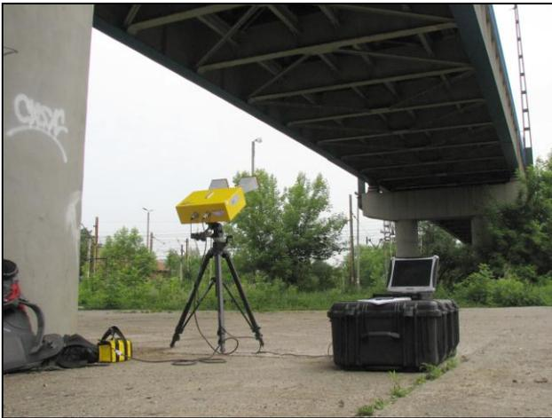
Figure 1. IBIS-S radar during work
