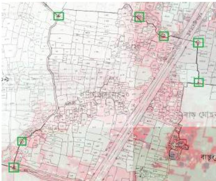
**Figure 3: Control point selection by edge matching**
