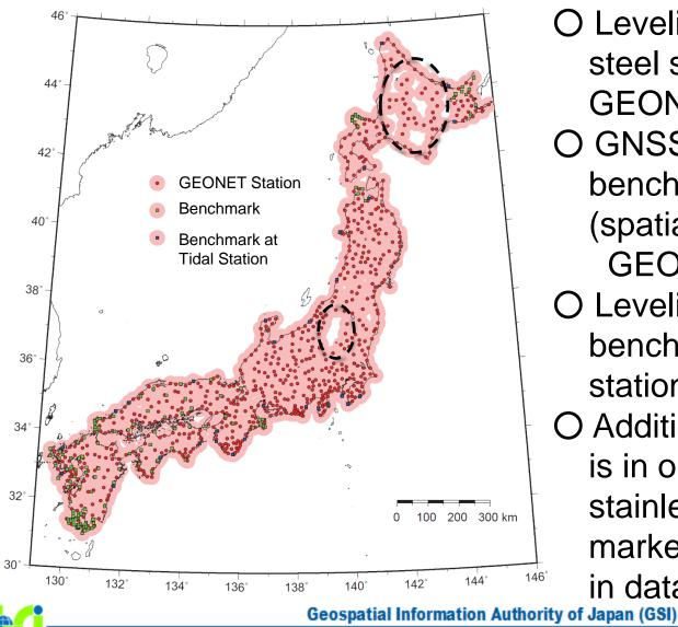
O Leveling survey on stainless steel survey markers at **GEONET** station: 775 O GNSS survey on benchmarks: 142 (spatially complement **GEONET** stations) O Leveling survey on benchmarks at tidal stations: 29 O Additional leveling survey is in operation on 35 stainless steel survey markers at GEONET station in data lacking areas.
