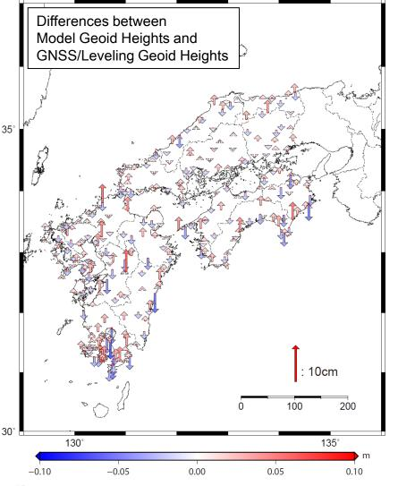
Geoid heights of GSIGEO2011 are compared with geoid heights determined by GNSS/Leveling to evaluate the consistency of the model with Japanese vertical datum.
