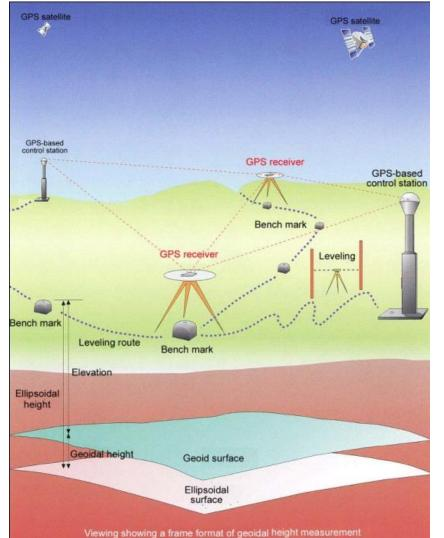
Geoid Height = Orthometric height - Ellipsoidal heights
