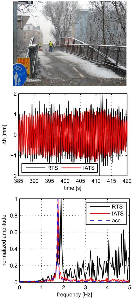
**Fig. 9** Excitation of the bridge by a single walker (top) and resulting height variations (middle) and frequency responses (bottom). Distance of IATS and RTS to respective targets: 33m. IATS observed natural features.
