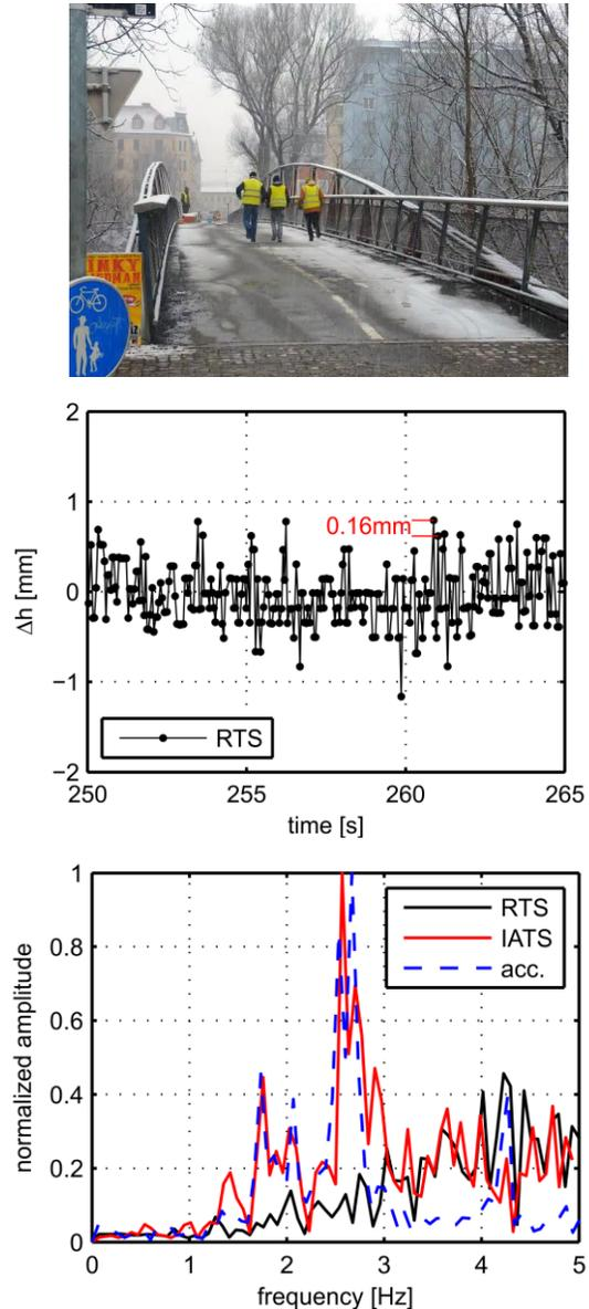
**Fig. 10** Excitation of the bridge by three runners (top) and resulting height variations (middle) and frequency responses (bottom). Distance of IATS and RTS to respective targets: 33m. IATS observed natural features.
