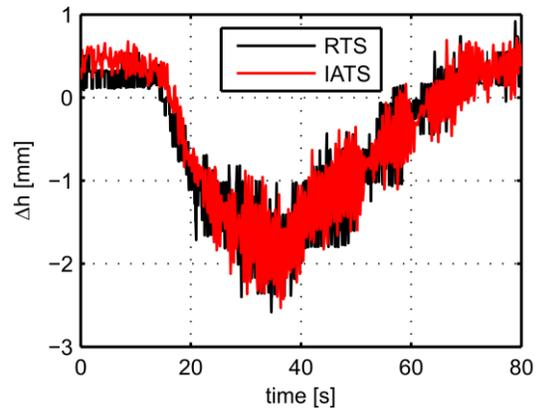
Fig. 12 Height variations due to vehicle crossing over the bridge. Distance of IATS and RTS to respective targets: 39m. IATS observed circular targets.
