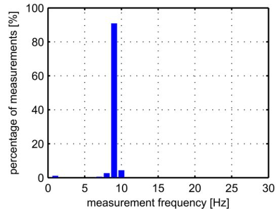
**Fig. 1** Distribution of measurement frequency of 1000 distance and angle measurements using a Leica TS15 total station locked onto a prism
