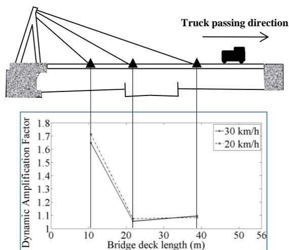
**Fig. 4** DAF values computed at the three GBMI targets for two passes of the test vehicle, at travel speeds of 20 km/h and 30 km/h. (GBMI targets shown in triangles).
