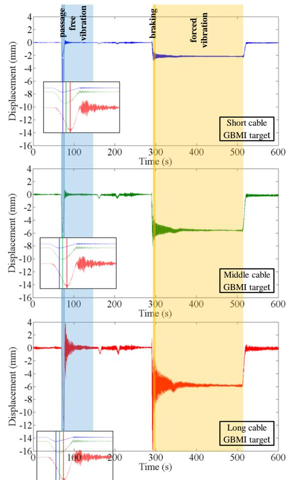
**Fig. 3** Dynamic displacements observed using the GBMI unit at the bridge deck realized at three locations, by the short (top), middle (middle) and long (bottom) cable anchor points.
