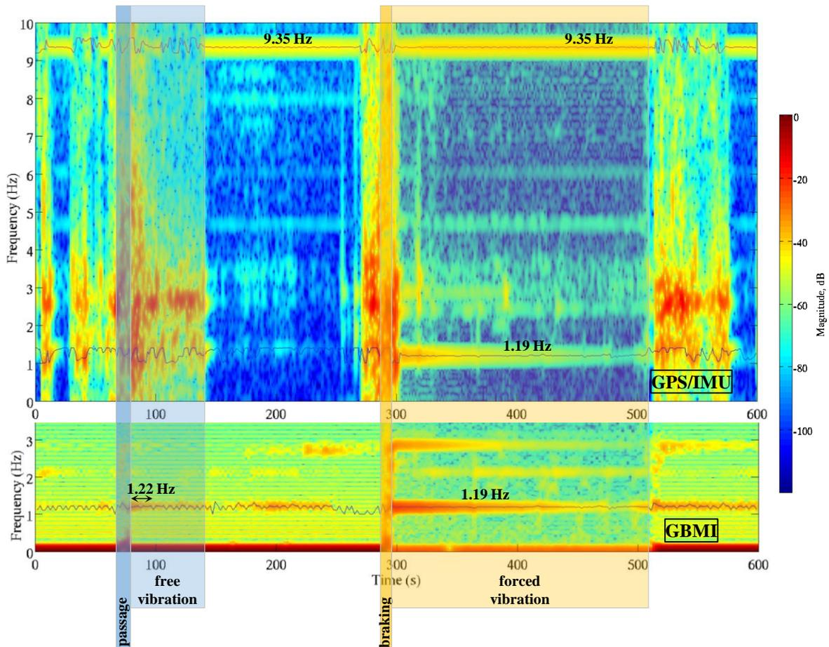
**Fig. 5** STFT plots obtained for the vertical acceleration of the vehicle (top) and dynamic settlement at the GBMI target at the deck by the long cable anchor point (bottom). The left part of the plot refers to a single passage of the vehicle at 20 km/h, whereas the right part shows an abrupt braking event.
