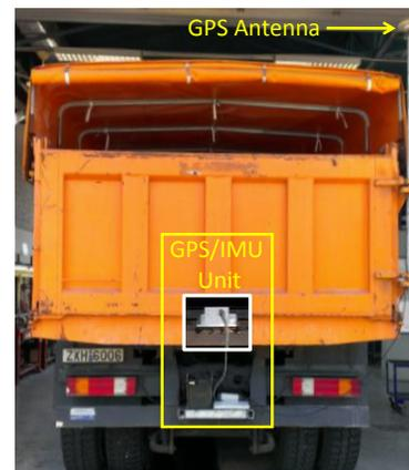
Fig. 2 Test vehicle with the GPS/IMU unit and GPS antenna fixed on it.
