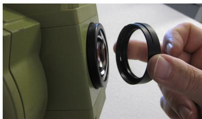
**Fig. 2** Divergent lens plugged on the objective.
