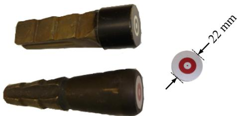
Fig. 4 Standard swisstopo target for dams.
