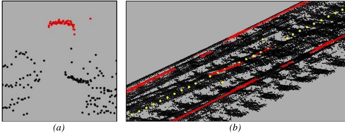
Fig. 11 Incorrect classification due to noise (a) and turnout (b)
