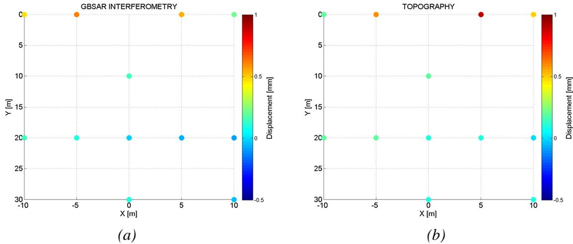
Fig. 3 Displacements measured at CRs location by GBSAR (a) and topography (b).
