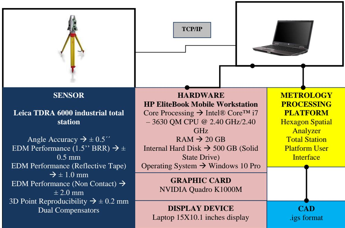
Fig.2: System architecture
