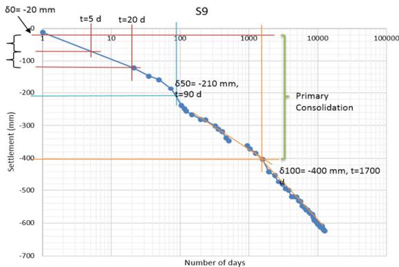
Figure 4(a). Settlement vs Number of Days (log scale for the x-axis) for control station S9
