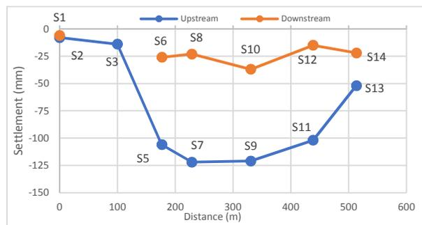
Figure 7. Observed settlement along the dam's upstream (blue) and downstream (orange) side of the crest on 24/02/1981
