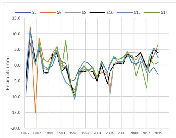
Figure 10(b). Residual settlements for control stations S2 – S14 along the downstream crest
