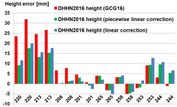
Figure 6. Errors at the control points between the reference heights and the measured heights from the point clouds.
