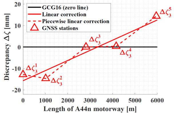
Figure 5. Linear and piecewise linear correction function for the GCG16 quasi geoid as a function of the length of the A44n motorway. The slope of the linear function is 4.9 mm/km.
