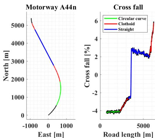
Figure 7. Cross fall of the eastern lane of the A44n motorway. Different draft elements can be distinguished.
