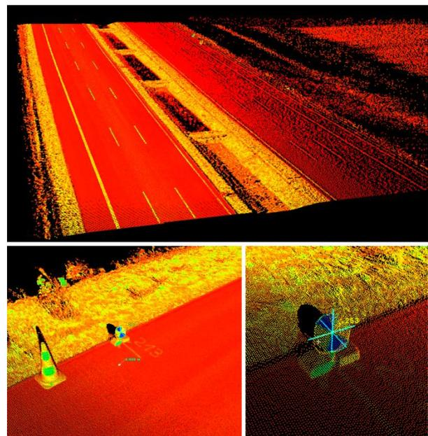
Figure 4. Point clouds of the Mobile Mapping System with a detailed view of a scanned control point (ID 253).
