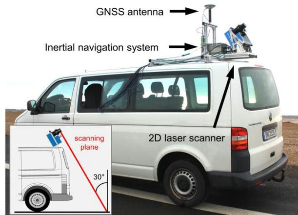
Figure 3. Mobile Mapping System for the acquisition of the road surface of the A44n motorway.
