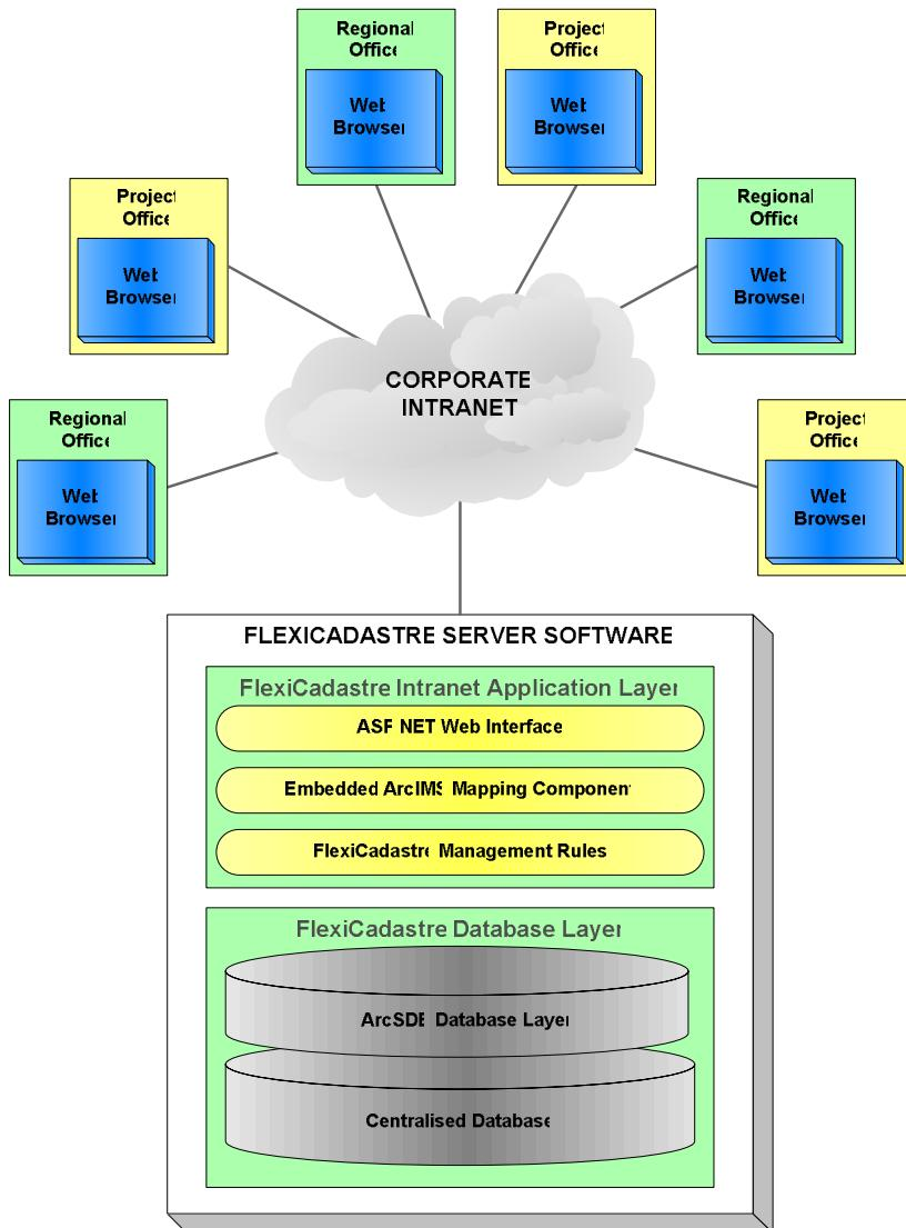
**Figure 3** FlexiCadastre High Level Database Design
