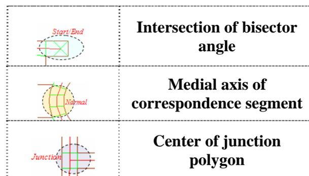
Fig. 7. Corridor centerline extraction
