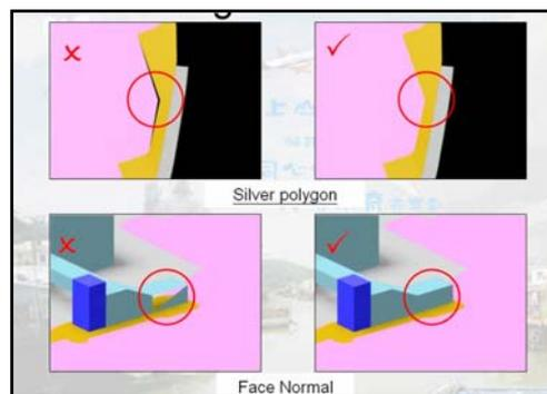
**Diagram (7): Common 3D Model Errors**
