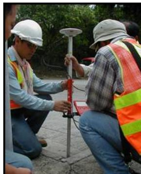
**Diagram (4): RTK-GPS Rover Equipment**
