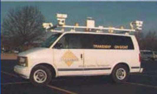
Vehicle-borne Laser Mapping System (VLMS)
