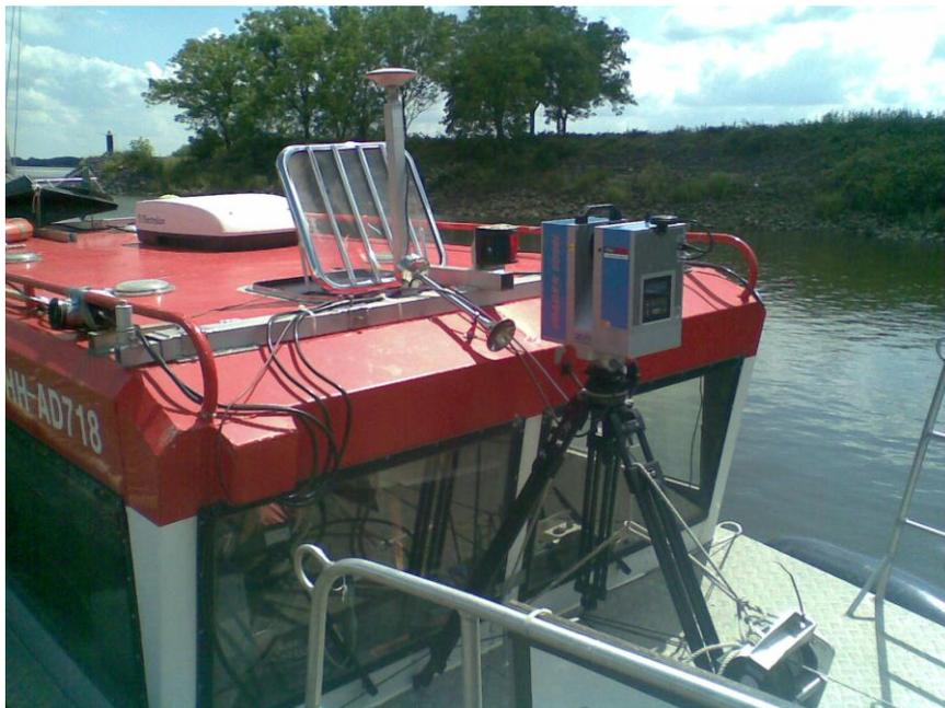
Figure 10: Installation of a terrestrial laserscanner from Zoller&Froehlich (owner: company DHPI) onboard the Level-A
