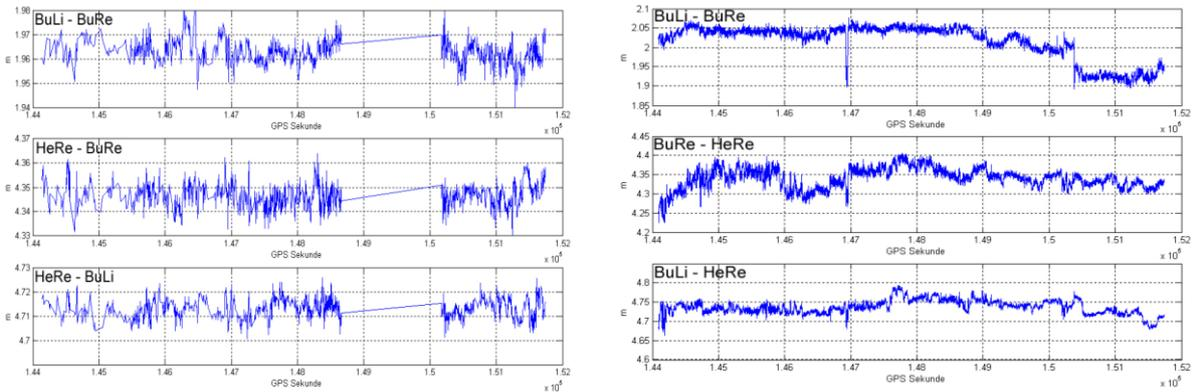
Fig. 2: Distances between GNSS antenna onboard the Level-A. Left: determined with RTK positions, right: determined with PPP positions. Different scales used.
