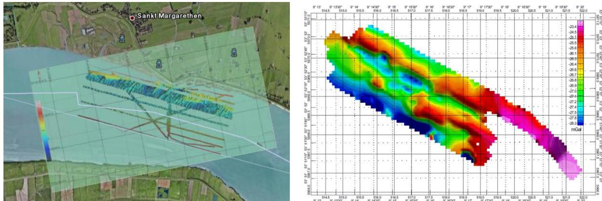
Figure 7: Profiles (left) and free air anomalies (right) measured with the HCU-HMSS and the gravimeter CHEKAN AM from Gravionic.
