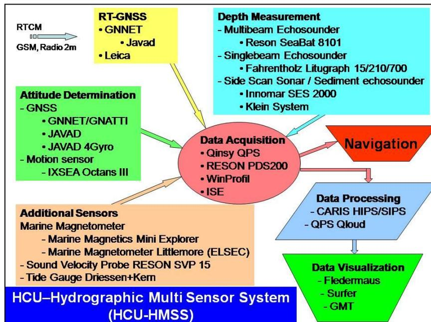
Figure 1: The HCU-Hydrographic Multi Sensor System
