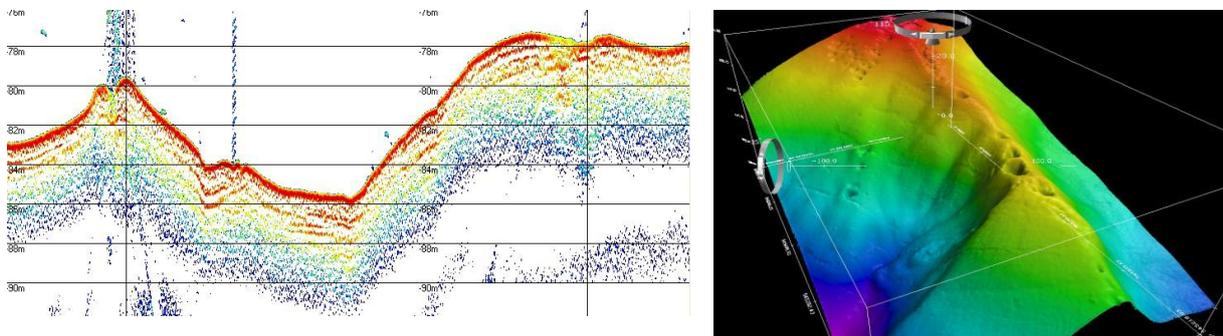
Figure 6: Pockmarks in the Lake Constance. Left: Subbottom profiling of active and inactive pockmarks, Innomar SES 2000. Right: Multi beam echo sounding DTM (from: *Böder and Wessel 2008*)
