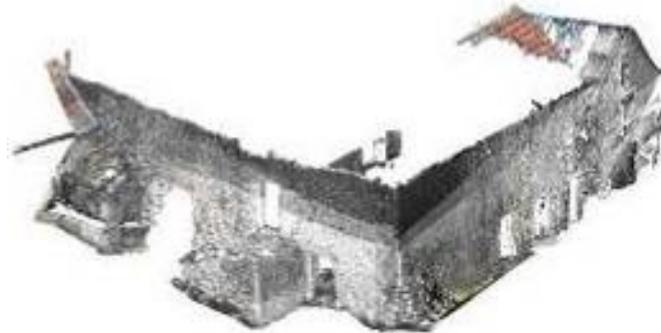
**Figure 3.3** Aligned and merged point clouds
