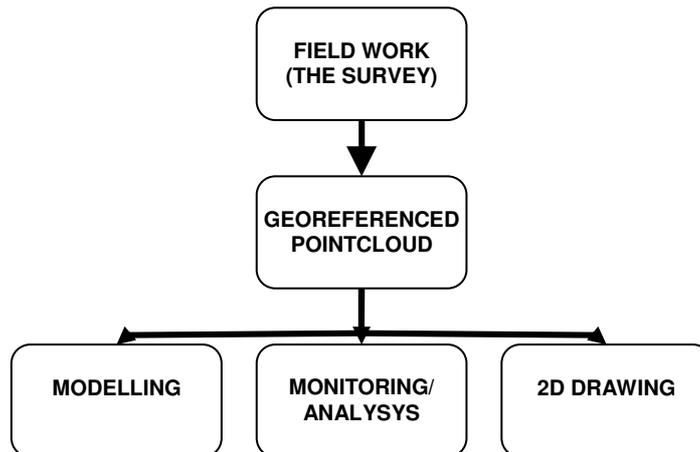
**Schematic view 1.1** 3D scanning processing steps
