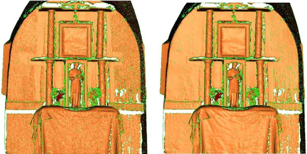
**Figure 3.6** Mesh after creation (left); Mesh after smoothing and noise reduction (right)
