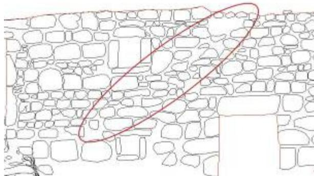
**Figure 3.8** Traces of a former roof
