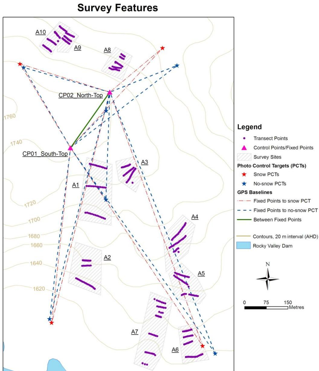
Figure 4: Survey features, transects, photo control locations for snow and no-snow photography capture, control mark locations and acquired GPS baselines.
