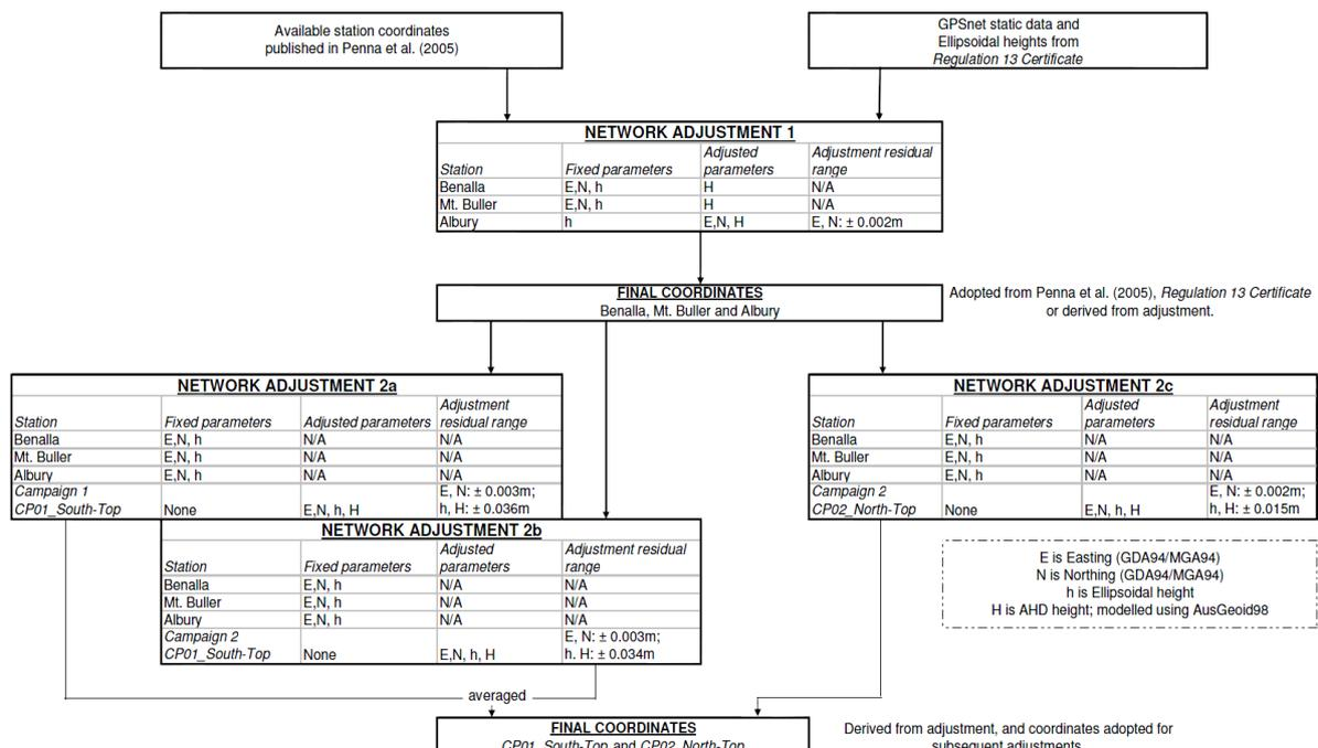
Figure 6: *Network Adjustments 1 and 2 (a, b and c)*, merging of survey control points into Land Victoria's GPSnet using network adjustments.
