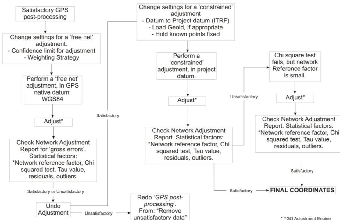
Figure 5: Network adjustment flow-diagram.
