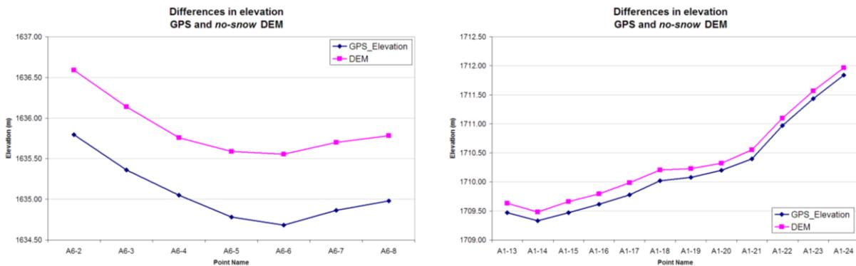
Figure 9: (a) (left) Survey site A6, 36 m transect and approximately 6 m between points and (b) (right) Survey site A1, 66 m transect and approximately 6 m between points.
