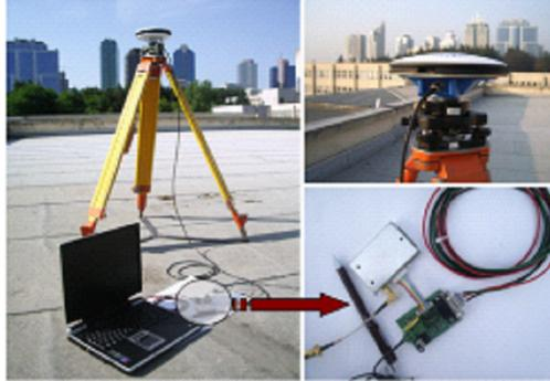
In this way, GPS data were collected by the OEM and geodetic receivers under the same conditions, which allows for precise assessment of the low-cost system.
