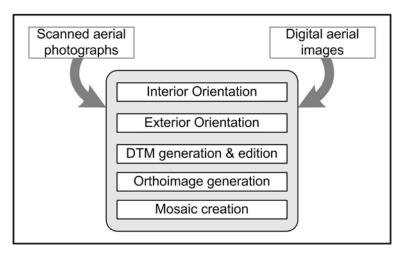
Figure 1. Orthoimage generation process
