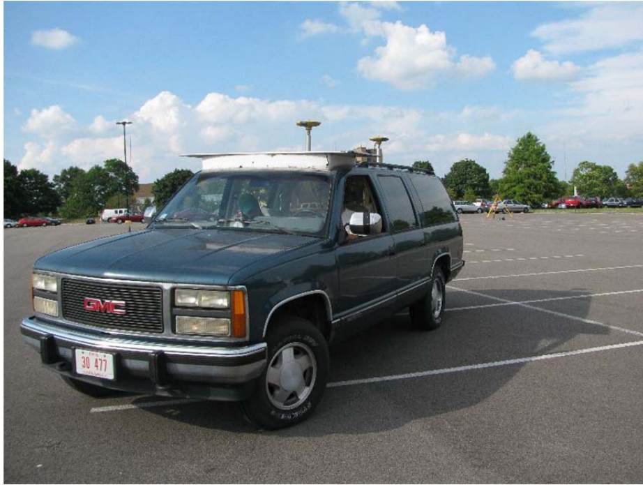
Figure 3: GPSVan in field tests at OSU Campus; note a GPS reference station in the back.
