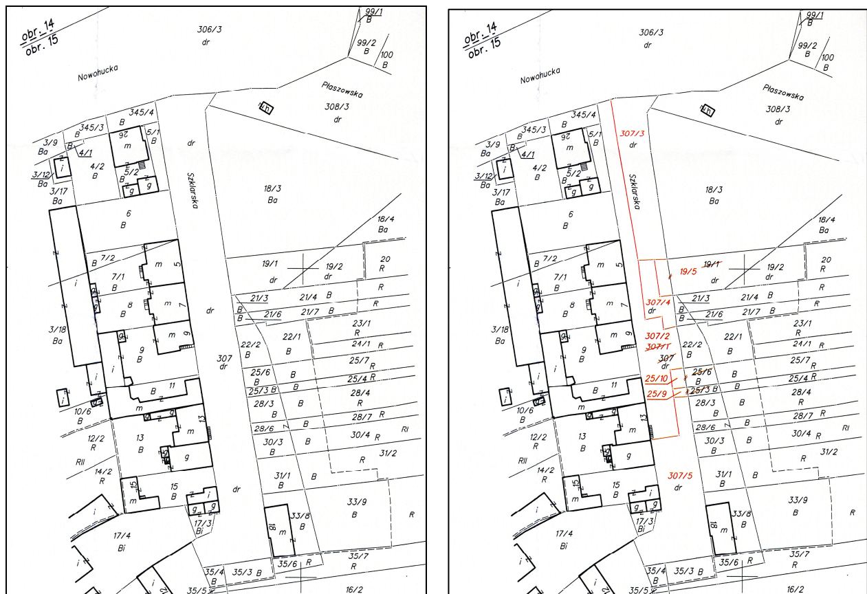
Figure 4. Condition disclosed in the land register and a map presenting the division of the properties connected in a record parcel.
