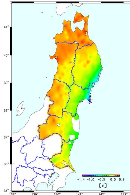
Fig. 5 Correction parameters developed for elevations
