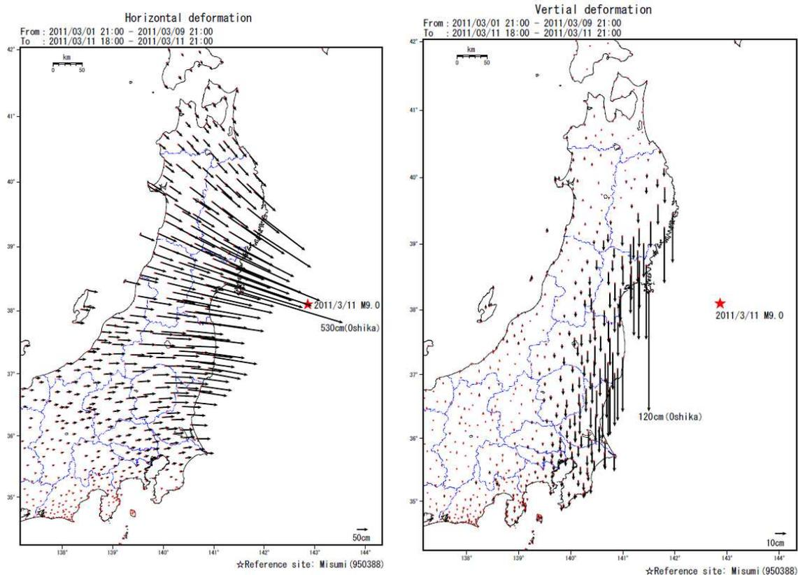
Fig. 1 Crustal movements caused by the 2011 off the Pacific coast of Tohoku Earthquake (Left: horizontal deformation, Right: Vertical deformation)
