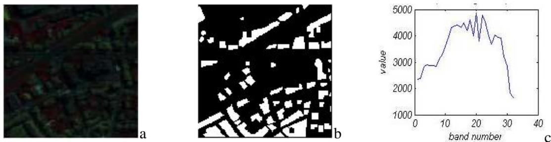
**Figure 2:** (a) the false color CASI image of study area ( $R=0.914$ ,  $G=0.620$ ,  $B=0.451$ ), (b) Ground truth data for accuracy evaluation, (c) The extracted spectra of building material
