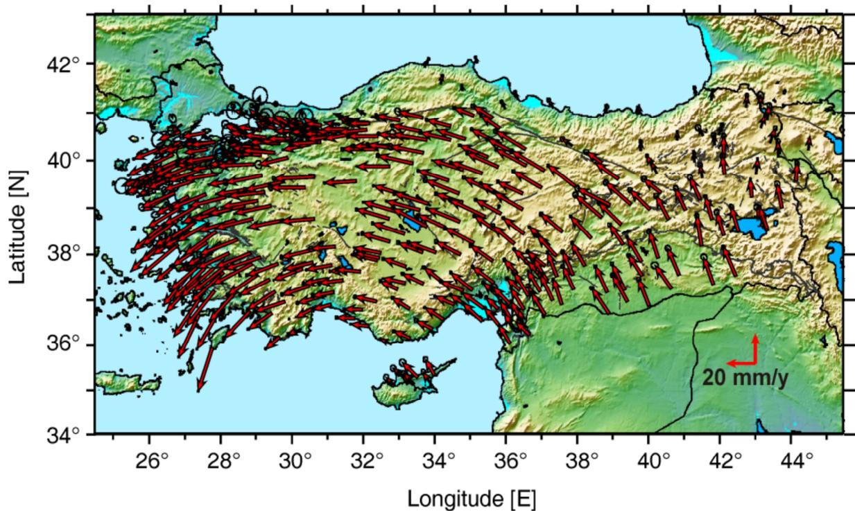
**Figure 5.** Horizontal Velocity field in a Eurasia-Fixed Frame using residual velocities of 17 IGS sites in Eurasia (ellipses are at 95% confidence level).(Aktug et al., 2009)
