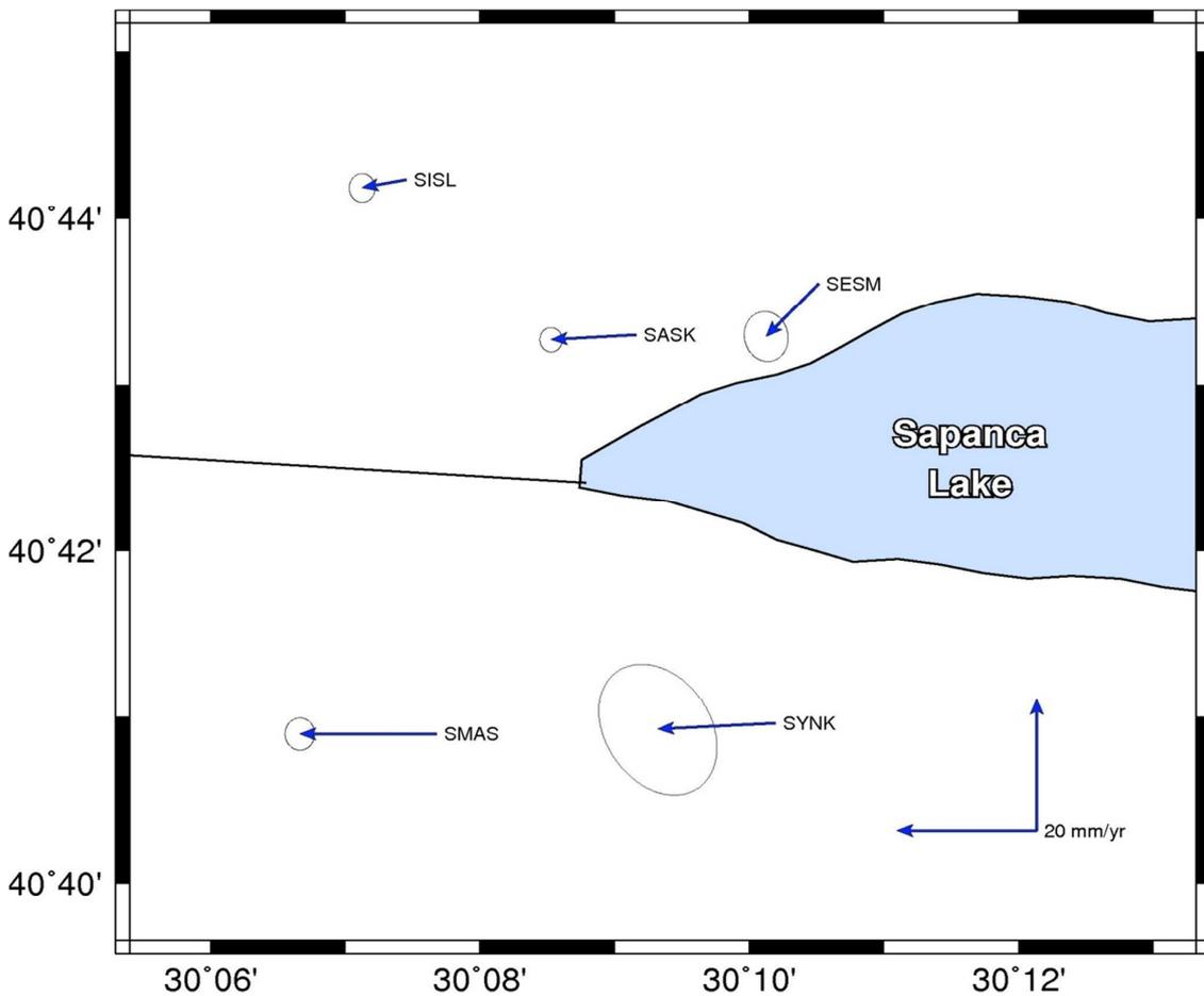
**Figure 4.** GPS horizontal velocities and their %95 confidence ellipses in a Eurasia-fixed reference frame for the period of 2005-2010
