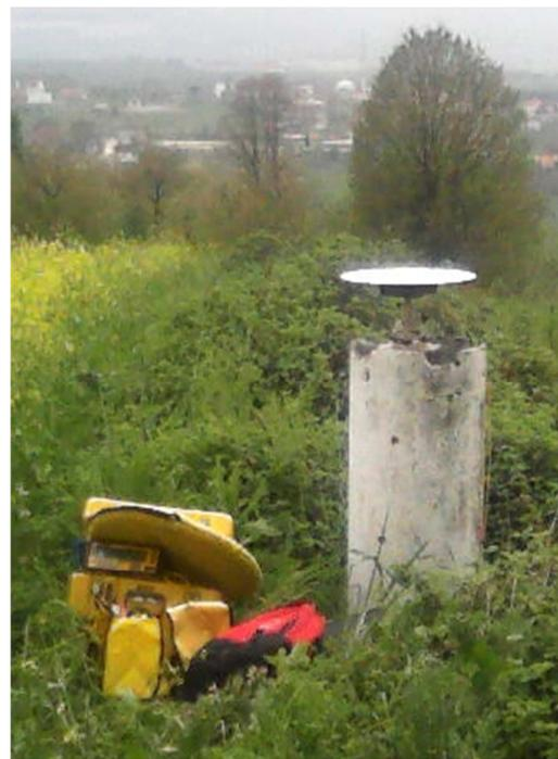
**Figure 2b.** Pillar used at SISL point
