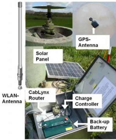
**CabLynx router including u-blox Lea-6T receiver, ANN-MS antenna and shielding, WLAN antenna, solar pannel, charge controller and battery.**
