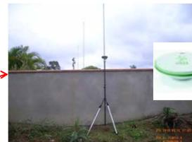
The tracking of the points was done with a Leica Geodetic GNSS receiver. This equipment is dual frequency (L1/L2). The measurement was made on the carrier phase, differential or relative positioning. The survey method used was static.
