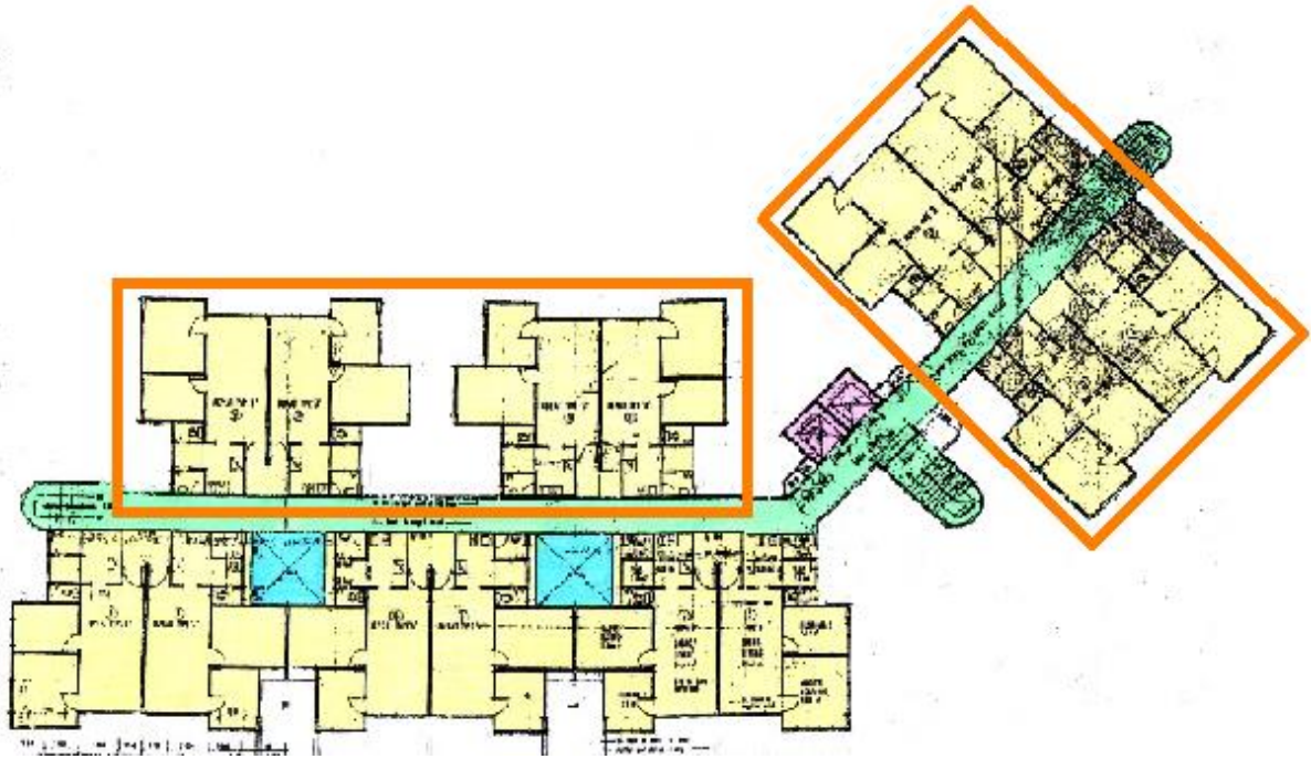
Fig 14 Single block with additional three (3) point blocks attached or linked by common corridors.
