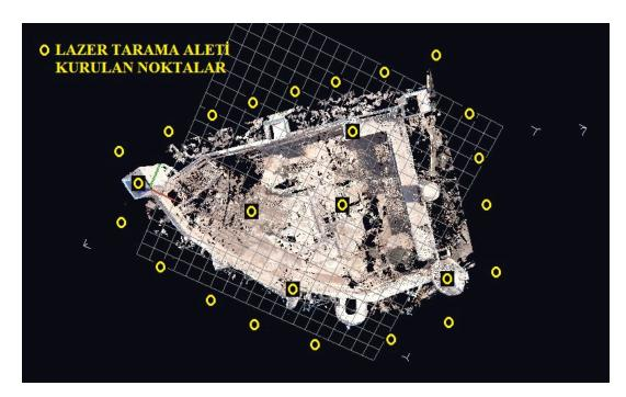
Image 12: Scanned Stations of laser scanning Trimble GX 3D
