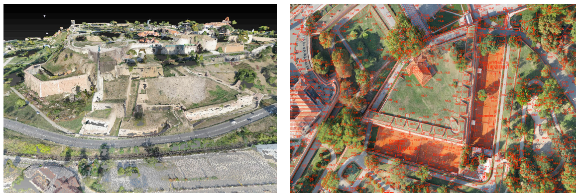
Fig.6. Point cloud (left) and ortho-photo map by using UAV technology overlapped with cadastral data for the location Kalemegdan fortress in Belgrade
