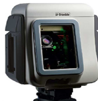
Image 4: Laser Scanning (Trimble GX 3D) used in work
