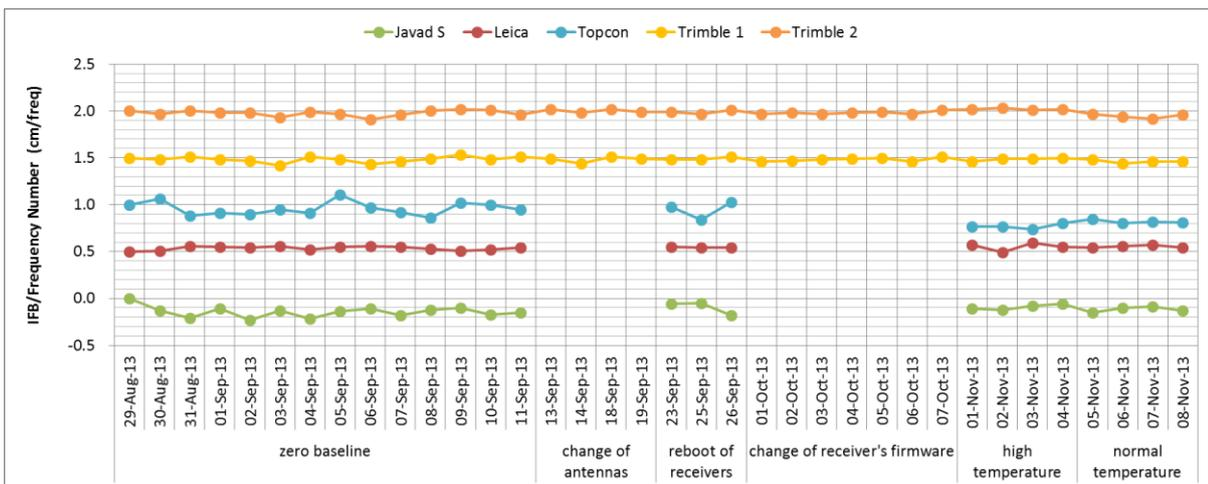
Fig.4: Variations of L2 IFB with respect to JAVAD DELTA receiver
