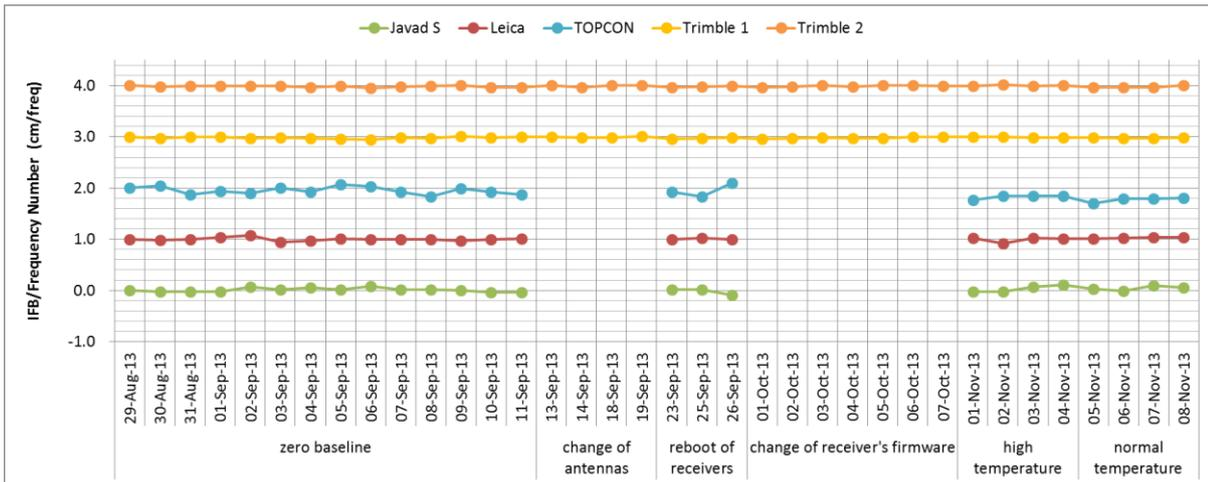
Fig.3: Variations of L1 IFB with respect to JAVAD DELTA receiver
