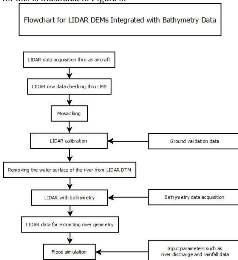
Figure 8 Workflow for LiDAR DTM calibration and bathymetric data integration
