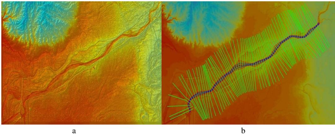
Figure 12 (a) Agno DTM with integrated bathymetric data and (b) extraction of river geometry using HEC-GeoRas in ArcGIS 10
