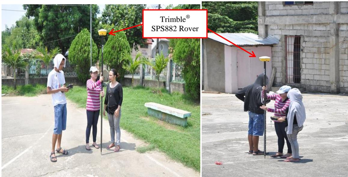
Figure 5 Validation points acquisition in Topo Surveying technique (UP-TCAGP, 2015, p.49)
