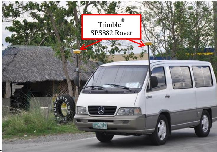
*Figure 4* Validation points acquisition in continuous topo mode (UP-TCAGP, 2015, p.50)
