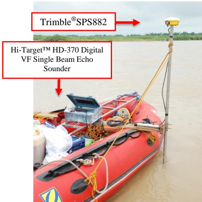
Figure 6 Bathymetric survey setup using a single-beam echo sounder (UP-TCAGP, 2015, p.53)
