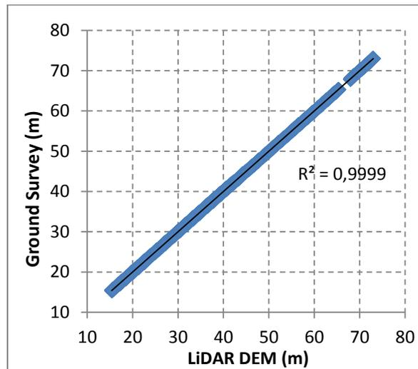
Figure 10 Correlation of LiDAR DTM and validation points acquired
