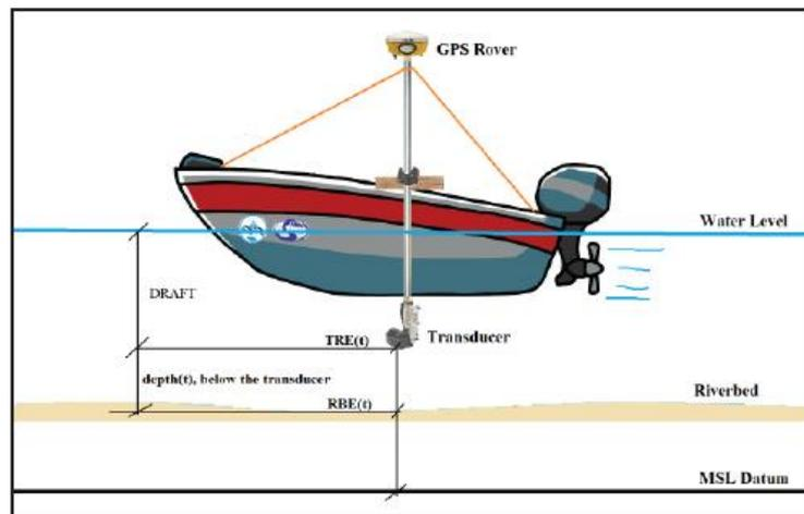
Figure 7 Echo sounder and GNSS rover setup (UP-TCAGP, 2015, p.30)
