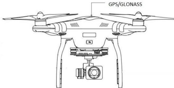
Figure 1. Position of GNSS antenna on DJI Phantom 3 Professional (customized from (DJI 2016)).
