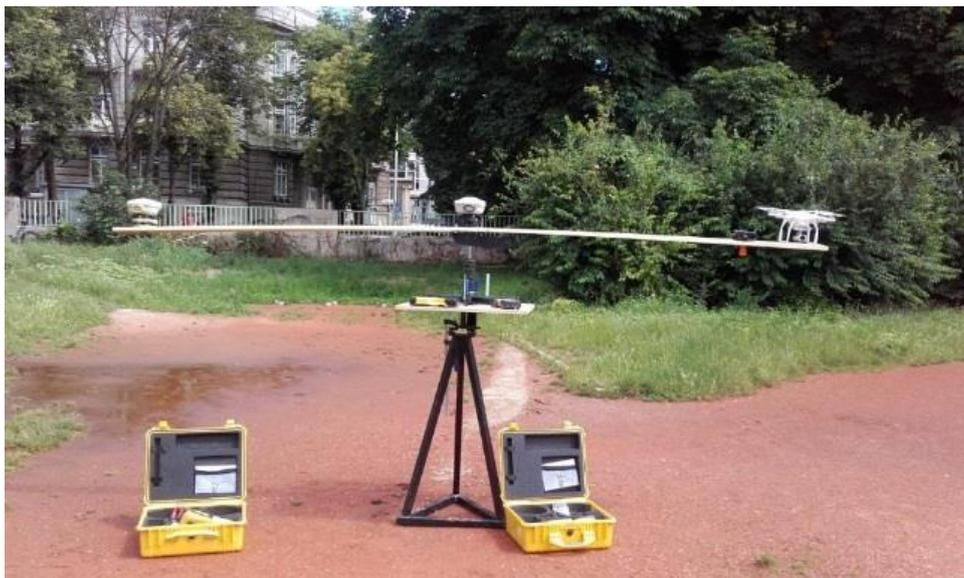
Figure 4. GNSS receivers Trimble R8 and DJI Phantom 3 Professional on the test platform.
