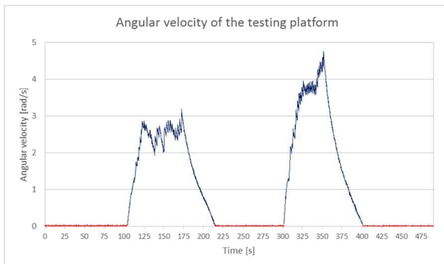
Figure 6. Angular velocity of the testing platform during kinematic test.
