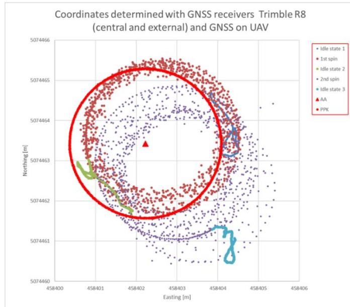
Figure 9. All coordinates determined during the kinematic test (GNSS receivers Trimble R8 (central and external) and GNSS on UAV).
