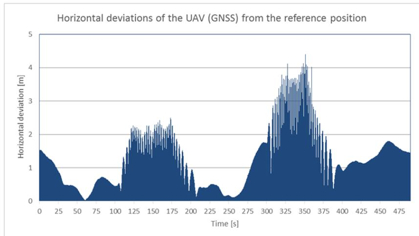
Figure 8. Horizontal deviations of UAV (GNSS) results from the reference positions.
