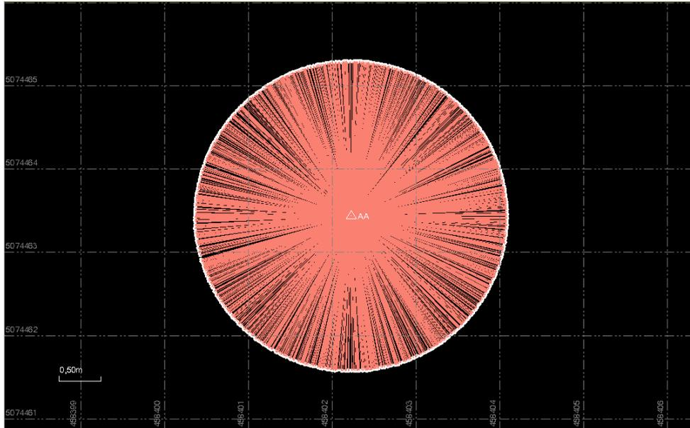
Figure 5. Circular trajectory of the GNSS receiver set up at the end of the testing platform (external GNSS receiver); central GNSS receiver is labeled with AA.
