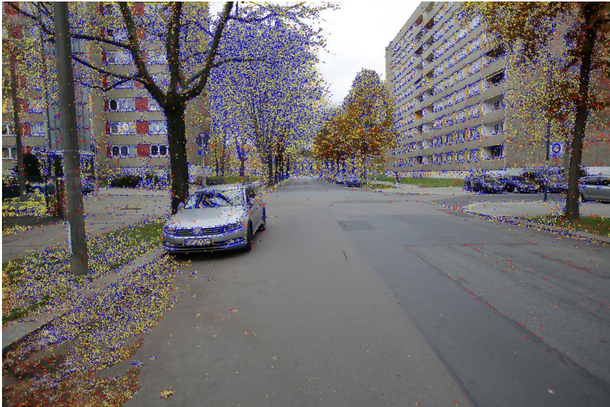
Fig. 3: Feature point detection on road. Feature points in red are detected by Colmap in yellow by openMVG and in blue by regard3D
